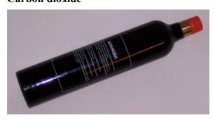
Because CO<sub>2</sub> becomes a liquid when compressed, it must expand to a gas in order to be used by the paintball marker. This expansion requires energy, causing the tank to cool as heat is used to expand the liquid CO<sub>2</sub> into gas. Eventually, under sustained fire and especially in cold weather, the tank can become so cold that ice crystals form on it. If the
